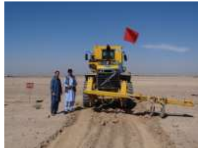
FEL with Ripper Attachment
