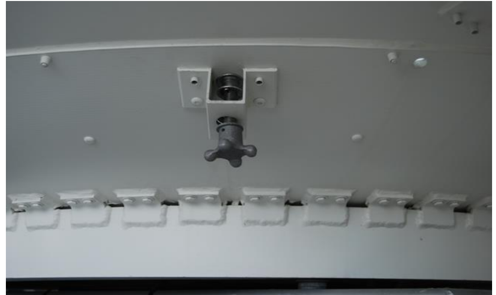
Reflector hold-down assemblies
